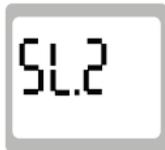
For 3-point calibration, the slope is first displayed for the lower, acid measuring range [SL. 1] and then for the upper, basic range [SL. 2].
