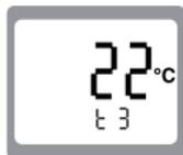
**Without temperature sensor: manual input of temperature of solution 3**
