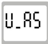
Asymmetry potential of the electrode at 25°C in mV
