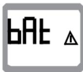
If the  $\Delta$  symbol appears together with „bAt“ in the lower section of the display, this means that the batteries are nearly empty and need replacing.
