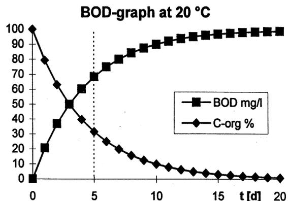
**Fig. 1:** Idealised BOD-graph at 20 °C (to HABECK-TROPFKE, 1992) compared with the proportional reduction in biodegradable organic compounds (C<sub>org</sub>). After 5 days incubation, approx. 70 % of the C<sub>org</sub> has been broken down: this is the equivalent of the BOD<sub>5</sub> value.
